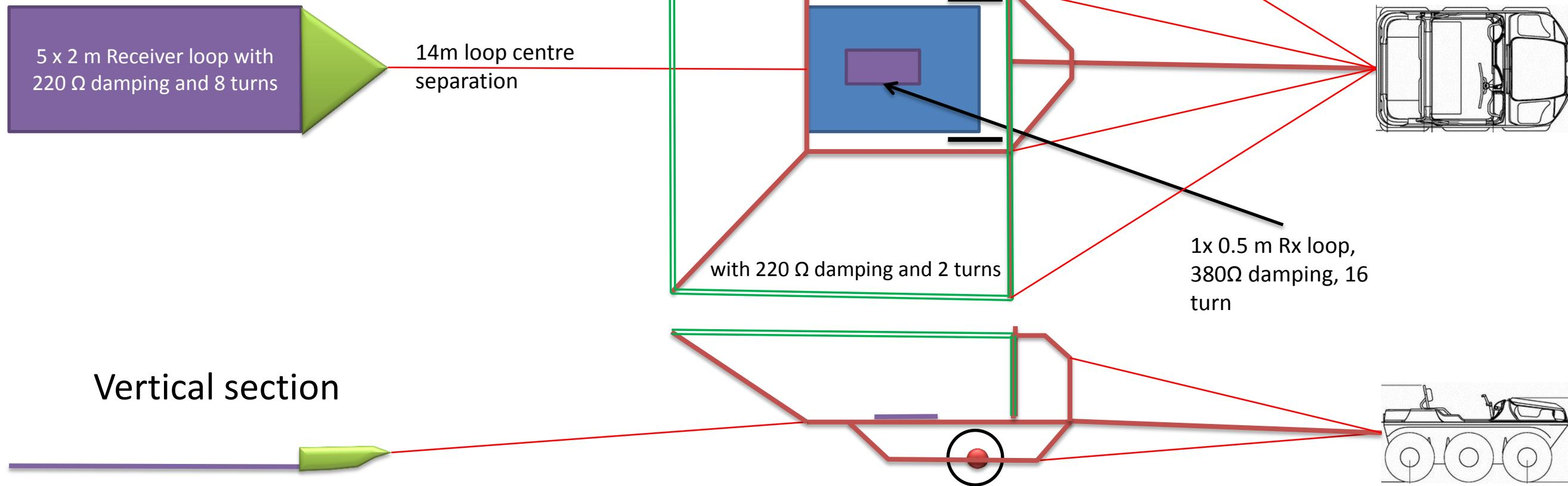
Transmitter loop suspension arms are attached elastically to prevent attrition upon impact with trees. Arms may be raised from the towing vehicle and fold inwards for obstacle avoidance and for compact transport when not surveying. The trailer draw-bar is detached for between-job transport. The trailer is lightweight and can be lifted by one person. Attrition is also avoided by addition of a breakaway pin.
