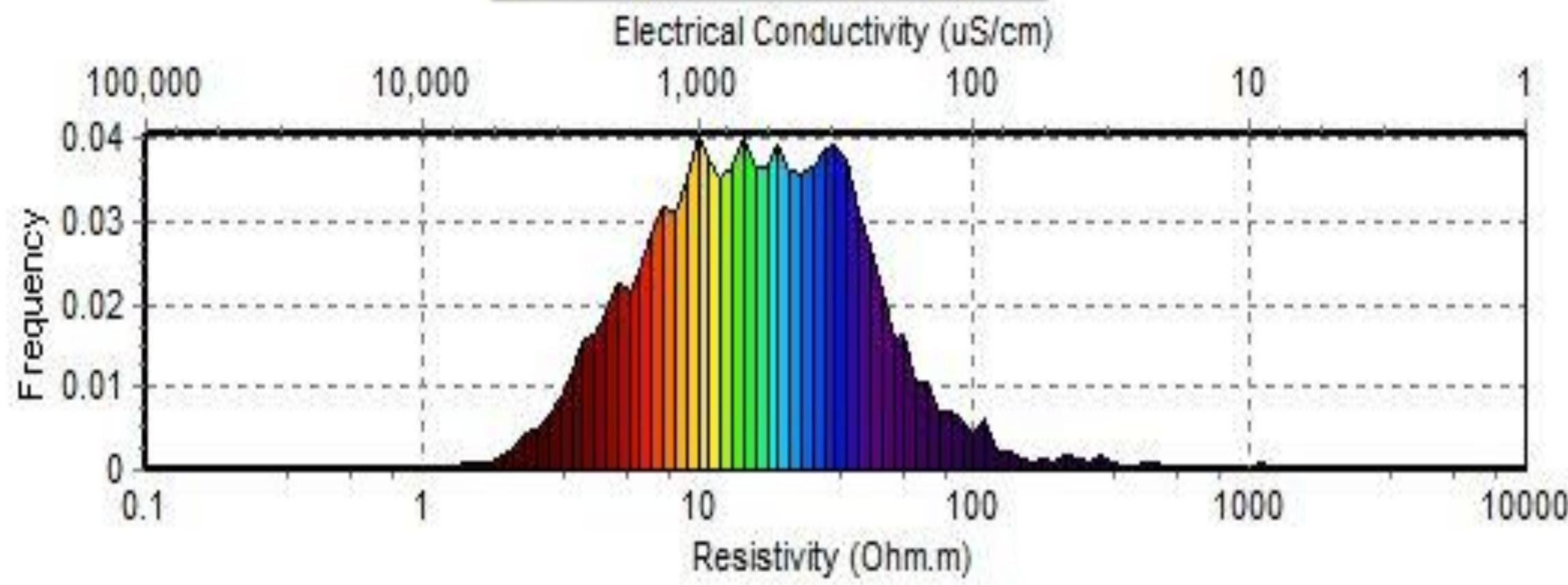
Observe that resistivities encountered span three orders of magnitude. The very high resistivities are somewhat artificially high due to the limitations of system response removal that presently exist with the system used.
