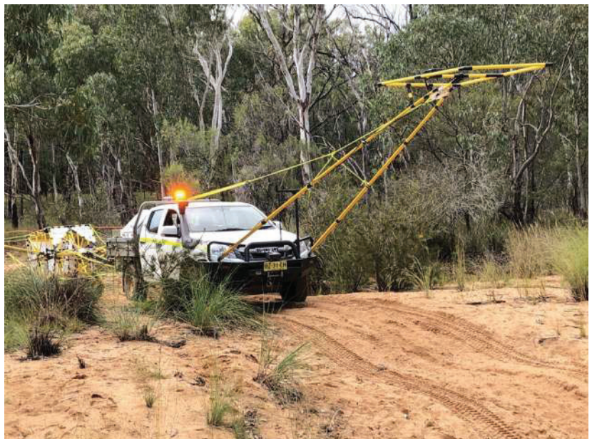
Figure 2. AgTEM front loop (Slingram) may be added as an option to create a second independent dataset.
