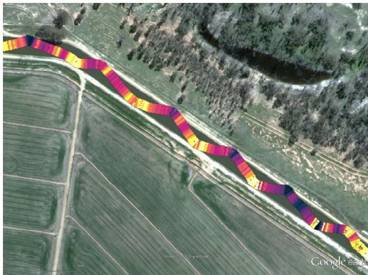
Figure 6: A sample of sludge thickness characterization using full waveform sonar. Conversion to actual thickness requires localized calibration.
