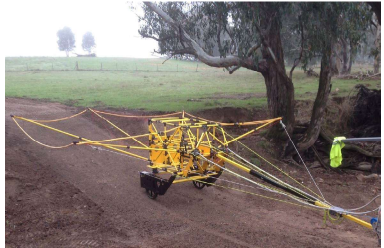
Figure 9: AgTEM towed transient electromagnetic system – an overview reveals the loop layout (the receiver loop is in the central plane).
