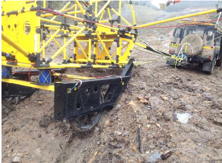
Figure 10: skid plates on the AgTEM-cart undercarriage and 600mm ground clearance permit traversing of exceptional terrain.
