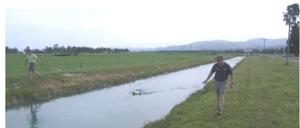
Figure 1 A Georesistivity meter, DGPS and sonar in a floating waterproof enclosure towing a submarine geoelectric streamer and towed by two walkers. Control and monitoring is via a WiFi link to the enclosure computer.
